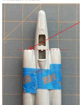
Assemble intakes first. Choose either standard cone or de-icer cone.
